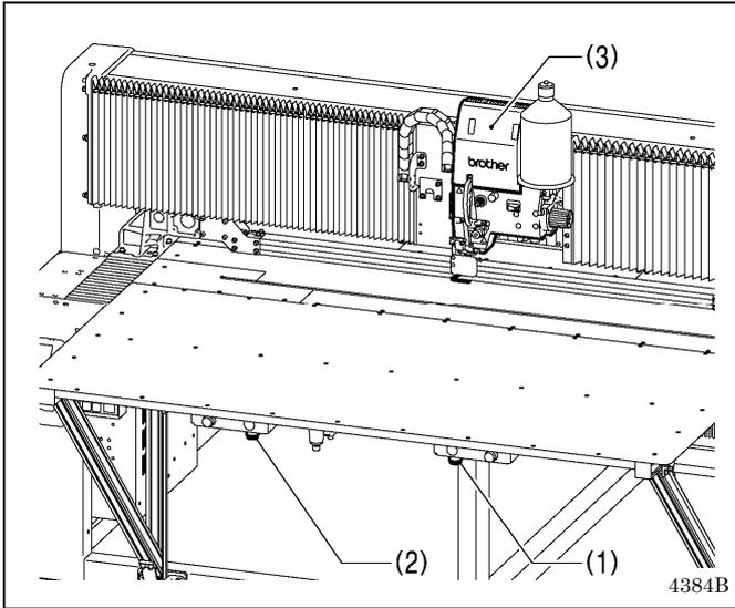
When the right switch (1) and the left switch (2) are pressed simultaneously, the machine head (3) will drop, and when the left switch (2) is pressed, it will rise. When the right switch (1) and the left switch (2) are pressed together while the machine head (3) is lowered, the sewing machine will start.
