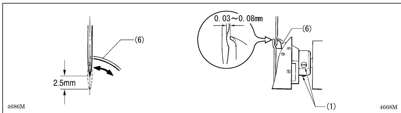
5. Adjust the position of the rotary hook so that the clearance between the needle and the rotary hook tip (6) is 0.03 to 0.08 mm when the rotary hook tip (6) is aligned with the center of the needle.
