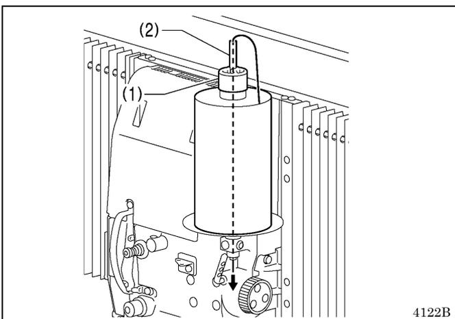
1. Set the thread spool in place, and then place the thread spool presser (1) against the top part of the thread spool to hold it in place.
