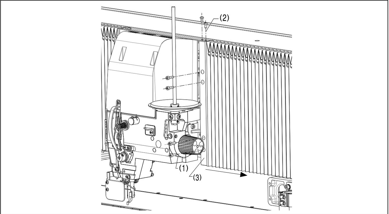
Remove the four socket bolts (1) and the two pan screws (2), and remove bellows bracket R (3) and move it in the direction of the arrow.
