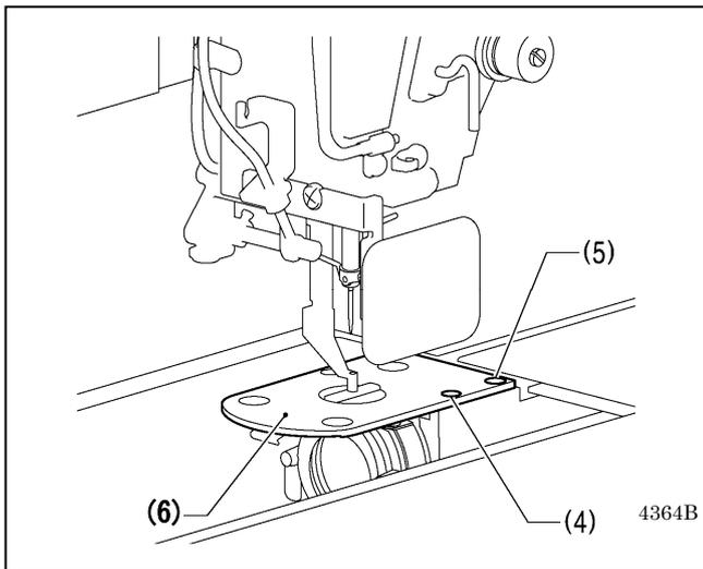
Next, remove the two screws (4) and the two flat screws (5), and then remove the needle plate (6).
