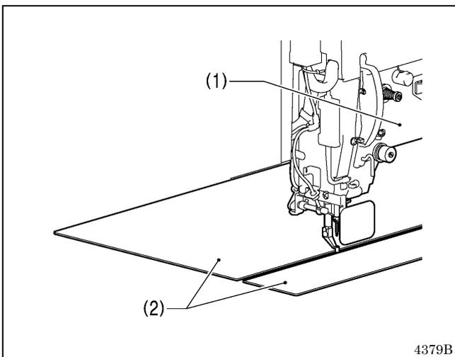
When carrying out adjustments in the area around the rotary hook, first switch the sewing machine to maintenance mode, and then move the machine head (1) to the left edge.
