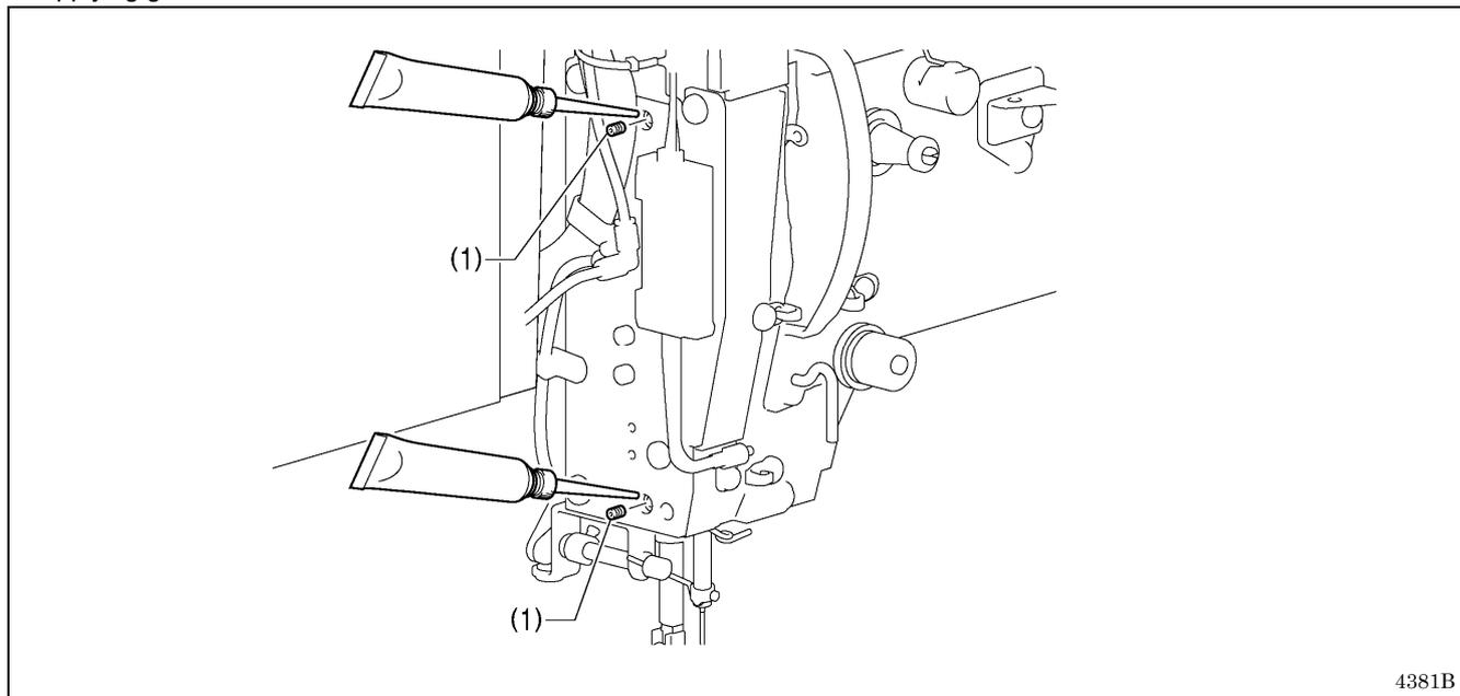
Remove the two set screws (1) from the two holes in the face plate, and apply grease to the holes.
