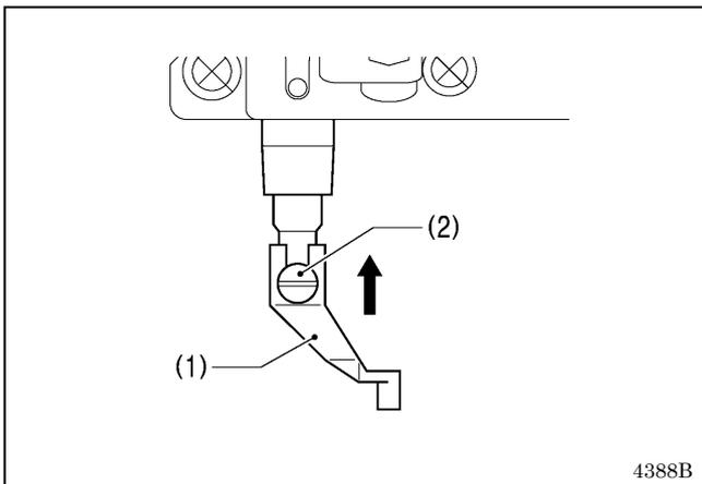
With the intermittent presser foot (1) pushed up to its highest position, install it with the screw (2).
