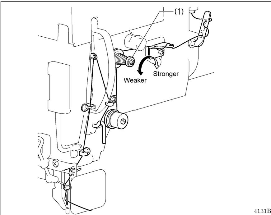
Use the digital tension to adjust the tension as appropriate for the material being sewn. (Refer to “Setting the tension value” below.)
