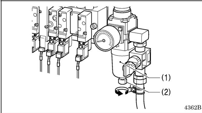
1. If water collects in the bottle of the regulator (1), turn the drain cock (2) in the direction of the arrow to drain the water.
