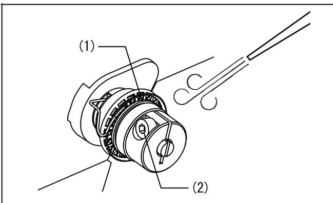
Use an air blower to clean the friction powder on the friction plate (1) about once a month.
