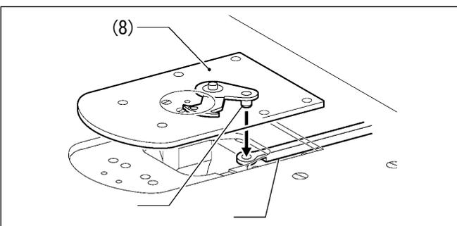
1. Apply grease to the pin (6), place it into the movable knife connecting plate (7), and install it to the needle plate (8).
