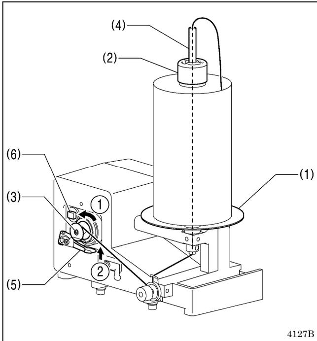
1. Place the thread on top of the thread spool bracket (1), and then place the thread spool presser (2) against the top part to hold the thread in place.
