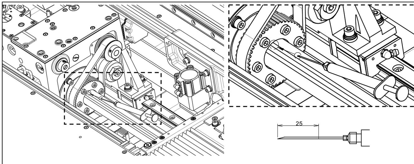
Insert the needle tip so that the sharpened point of the needle tip is in the groove of the spline shaft, and then apply 0.5 mL of grease.
