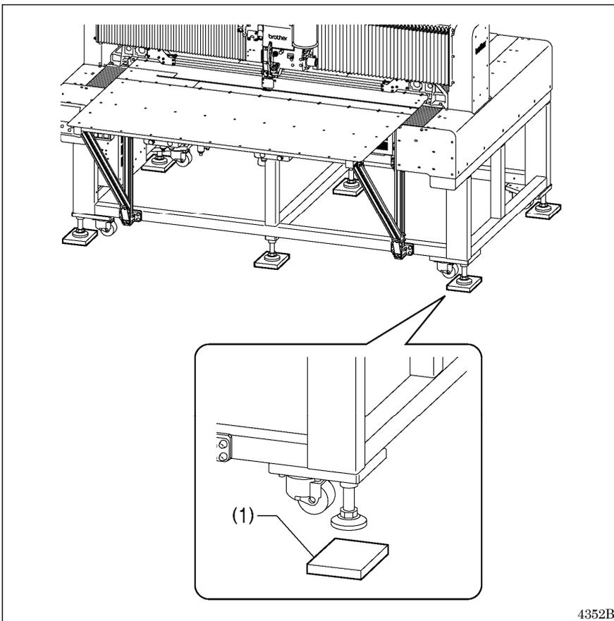
1. Place the sewing machine onto the rubber cushions.
