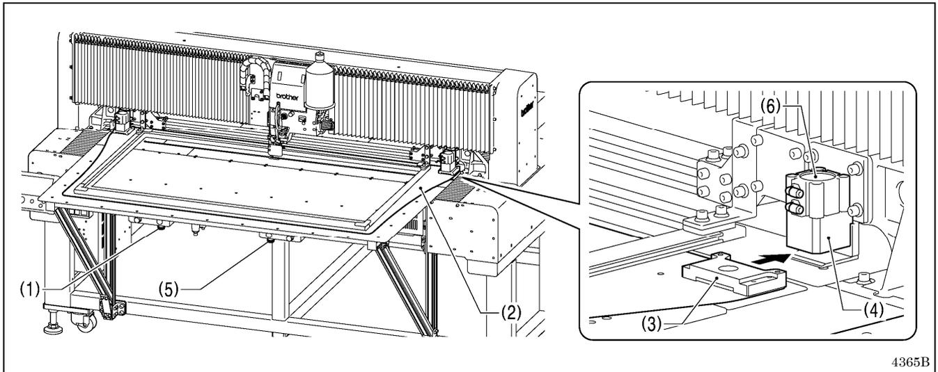
1. When the left switch (1) is pressed, the feed plate (2) will unlock so that it can then be removed.
