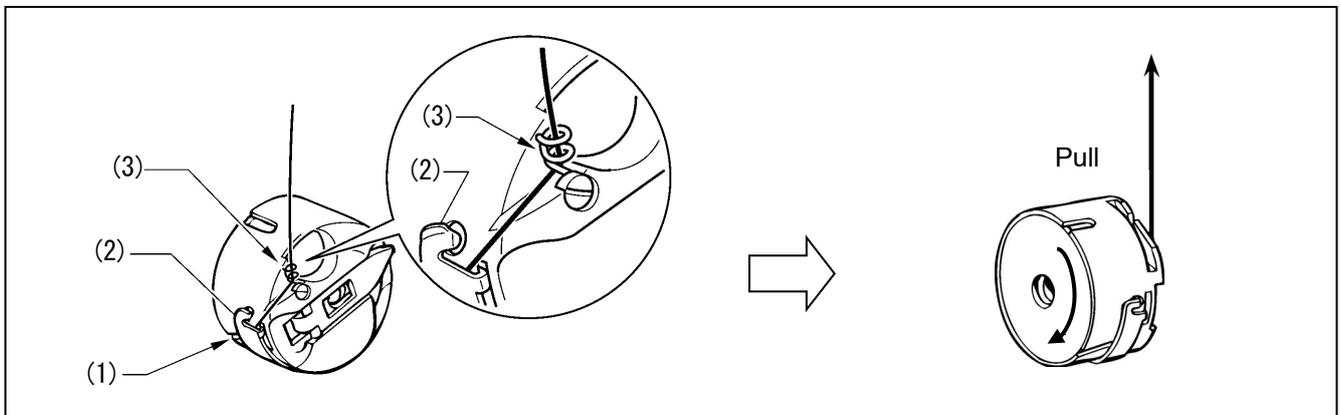
1. While holding the bobbin so that the thread winds to the left, insert the bobbin into the bobbin case.
