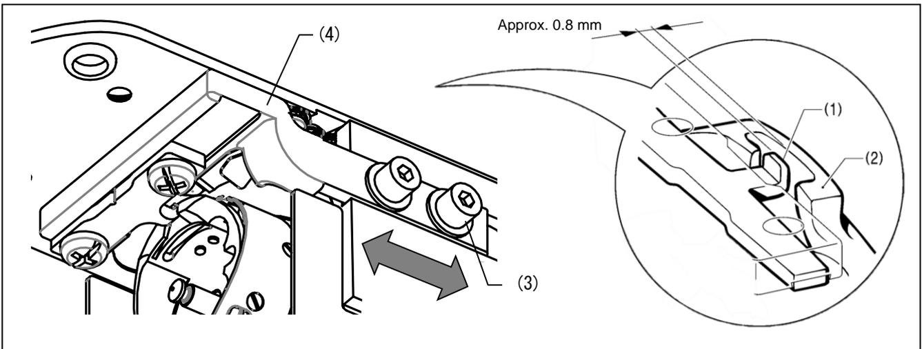
Loosen the two screws (3) and move the hook stopper setting base (4) to adjust so that the tip of the hook stopper (1) is approximately 0.8 mm away from the needle drop surface of the inner hook (2).
