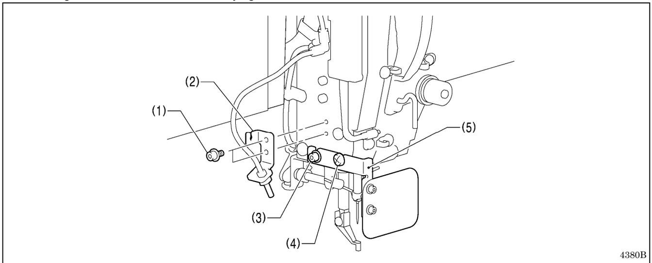
Loosen the two bolts (1), remove the needle cooler device (2), and then loosen the bolt (3) and the screw (4) and remove the eye guard assembly (5).
