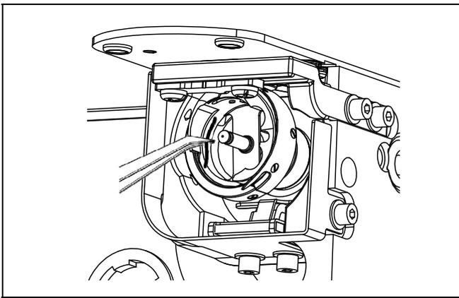
Remove the bobbin case, and then remove the dust and lint from around the shuttle.
