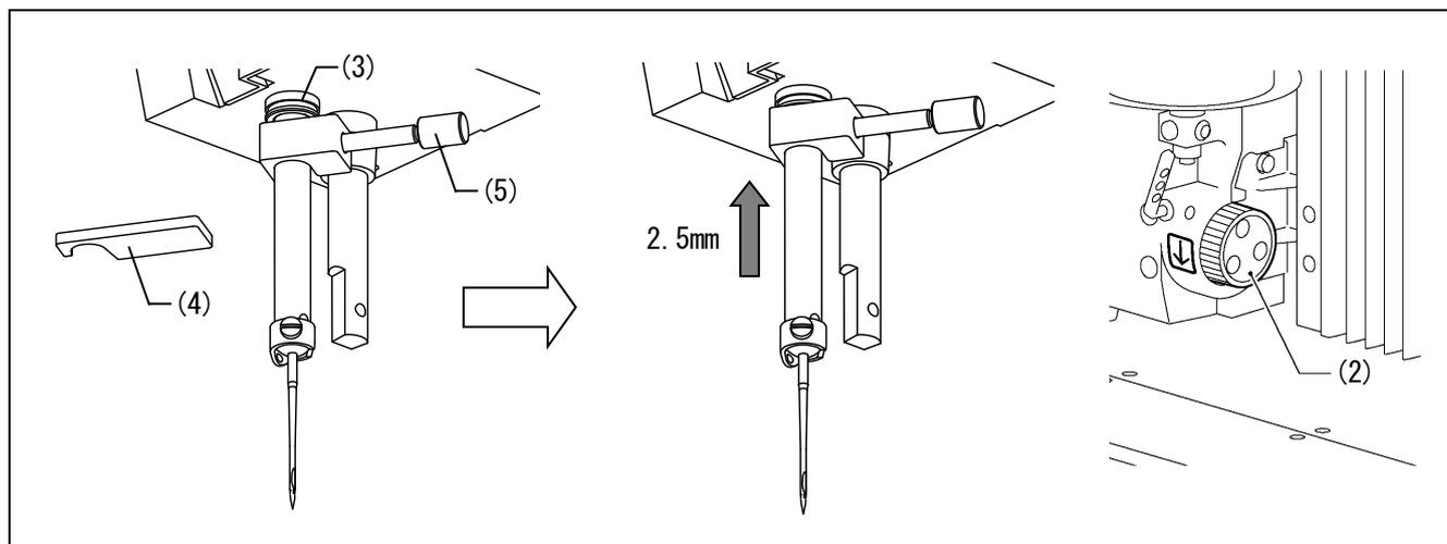
4. Remove gauge 1 (4) from the needle bar, and then turn the pulley (2) in the direction of the arrow so that gauge 2 (5) is against the bottom of the needle bar bush (3).
