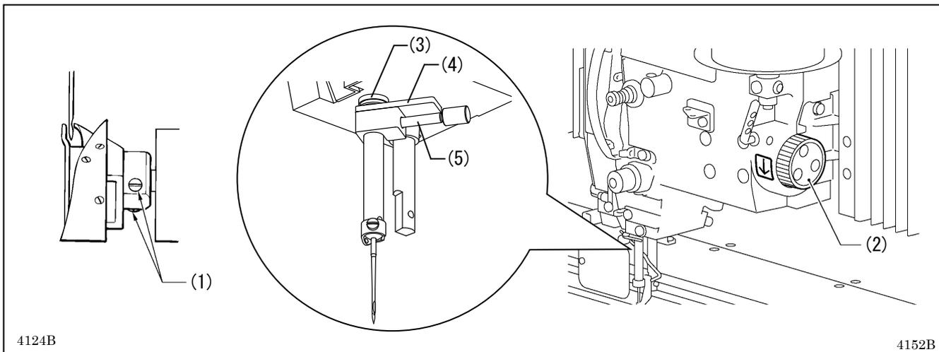
Use the <Gauge 1 (SC4846-001)>, <Gauge 2 (SC4847-001)> and <Knob screw M4 (SC4845-001)> specified by Brother as the gauge 1 (4) and gauge 2 (5).
