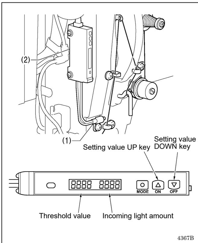
1. Thread the upper thread and pull the upper thread straight.
