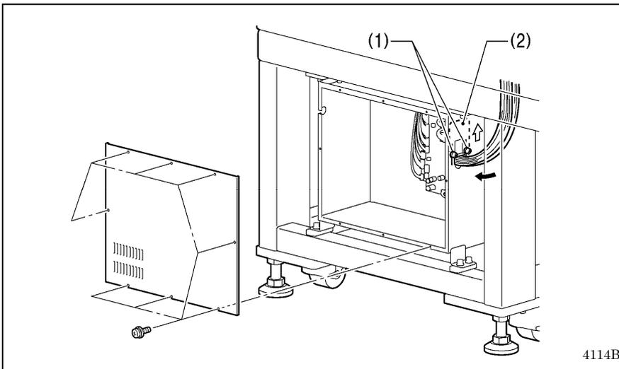
1. Remove the cover of the control box.
