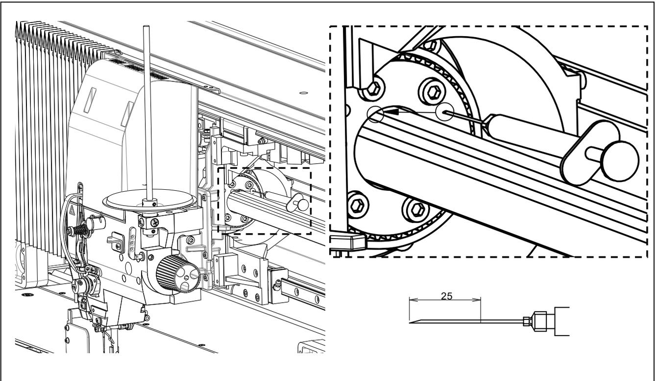
Insert the needle tip so that the sharpened point of the needle tip is in the groove of the spline shaft, and then apply 0.5 mL of grease.
