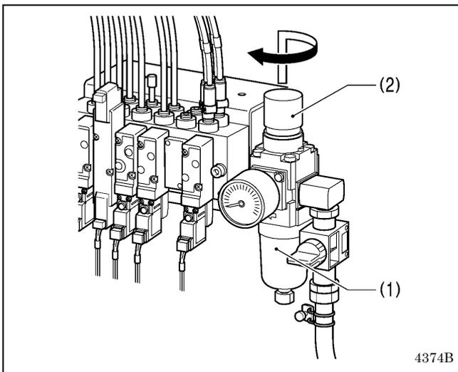
Lift up the handle (2) of the regulator (1) and then turn it to adjust the air pressure to 0.5 MPa.
