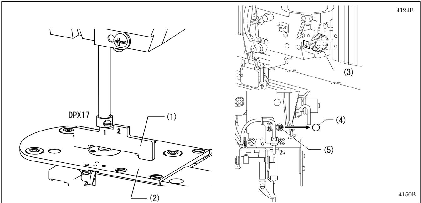
Use the <Needle bar height tool RH (SC0798-001)> specified by Brother as the needle bar height tool (1).
