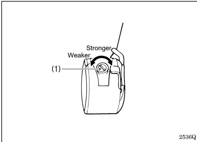
Adjust the thread tension to the weakest possible tension by turning the thread tension nut (1) until the bobbin case will not drop by its own weight while the thread end coming out of the bobbin case is held.
